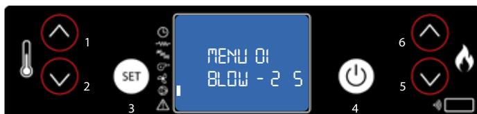
3. Set the speed using the button 1. With key 1 you set the speed of the fan.
