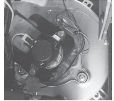
**Flue gas temperature sensor:** thermocouple that measures the temperature of the fumes while keeping the operation or shuts the thermostove when the flue gas temperature drops below the preset value.
