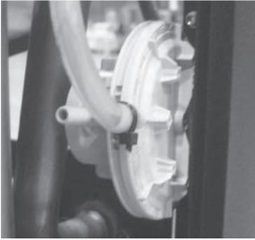
**Pressure switch:** monitors depression in the smoke duct. It is designed to shut down the pellet feed screw in the event of an obstructed flue or significant back-pressure in the presence of wind. At the time of the pressure switch will show **"ALAR-DEP-FAIL"**.
